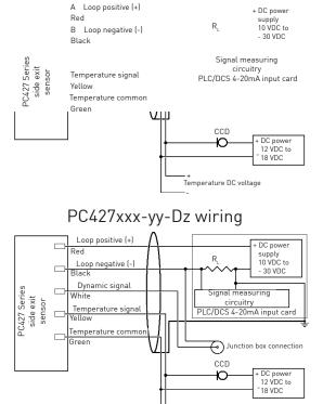
All wire and cable used for installation of the PC425 Series sensor should be shielded. Generally accepted instrumentation wiring practice considers the best way to ground the shield is to connect it at only one end of the cable. The shield should not be wired to ground at both ends of the cable. The Wilcoxon PC427 Series sensor has the shield connected to the case at the sensor end of the cable.
