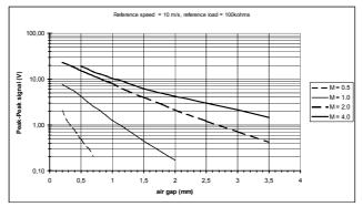
Typical signal amplitude with ferromagnetic gear. Surface Speed = 10m/sec (393.7 IPS) Load = 100 kOhm
