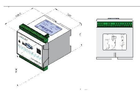
**Mounting** DIN-rail DIN 4622713 (EN 50022) or mounting plate DIN 43660 (46121)
